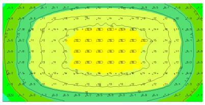
The above plot is a 6x12M area with 2x10M runs of AQF-050 Festoon on the long axis, spaced 3M apart.
